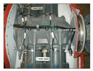
6. Attach the green ground wire to the engine (photo at right), and test the connection by checking for continuity between the engine and the ground pin on the plug.
