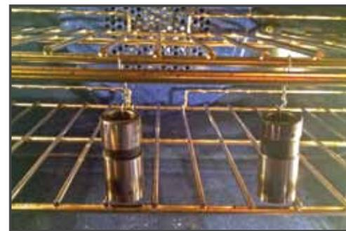
Oven used to "bake" the dry lifters.
