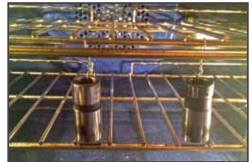
*Oven used to "bake" the dry lifters.*
