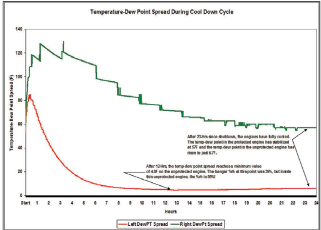
in the future, internal engine parts are coated in oil, therefore making the concern over internal relative humidity irrelevant. While I find this argument to be compelling, I know it is not consistent. There have been a few times since I've owned my airplane that it has sat for up to a month without flying, and without dehydrators (prior to 2006). The oil analyses after these periods confirmed that long periods of inactivity led to rust on the internal
