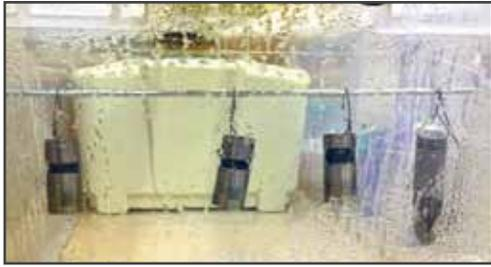
The high humidity chamber used for testing the lifters.
