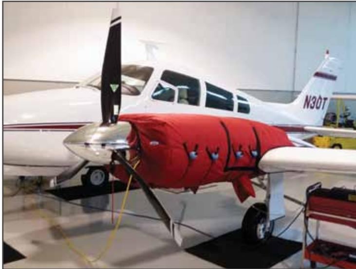
(Above) Engine blankets facilitate uniform engine heating as well as reduce condensation. (Right) Plugs for my exhaust augmenters completed the seal.
