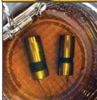
Above: The "fryers" used for "cooking" the lifters. The oil was heated to 190 deg. F. Left: Lifters suspended in the oil for one hour.
