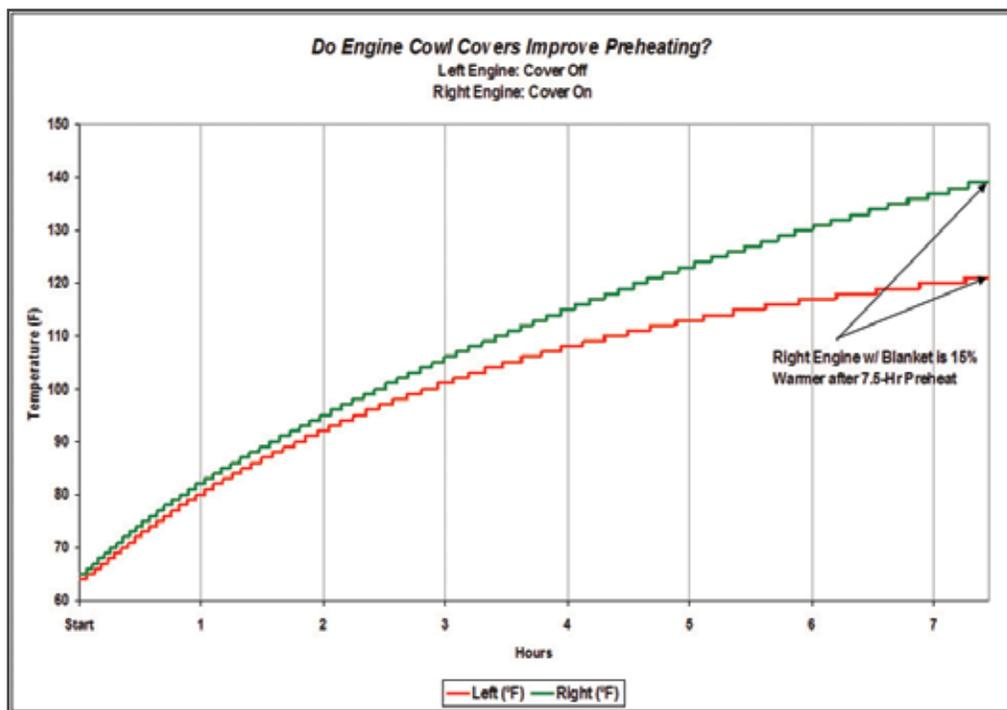
Bottom line: Kennon engine cowl covers allowed the Reiff engine heater to warm my right engine temperature 15% higher than the uncovered left engine. The final temperature was within 10% of my normal operating temperature.
