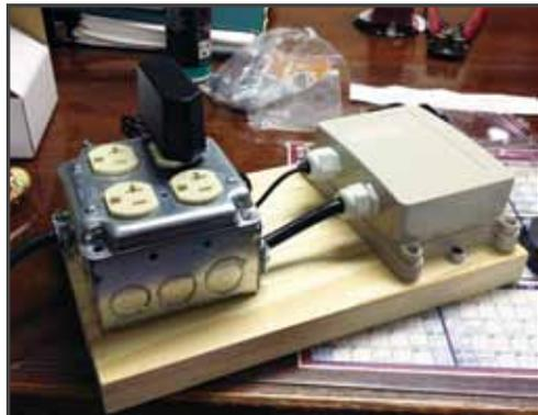
The GSM Auto switch allows me to turn my engine heaters on and off from my cell phone.
