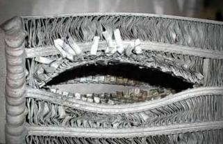
Although it's relatively rare, oil coolers can be damaged because of insufficient preheating.
